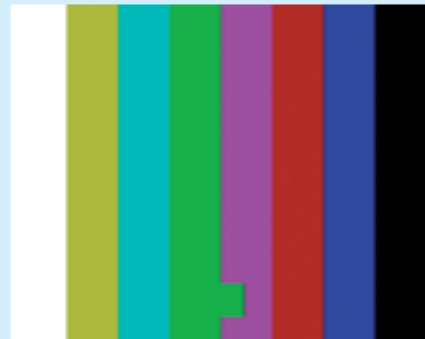
ITU-R BT.801-1 colour bar test pattern with moving element for automatic picture assessment during EMS measurements.
